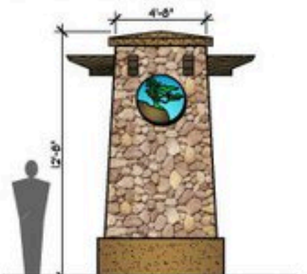
OPTION 'C' LARGE MONUMENT PILASTER (SECTION) (FIELDSTONE)
